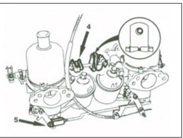
(a) Reconnect the mixture control wire with about 1.6 mm (1/16 in) free movement before it starts to pull on the jet levers.
