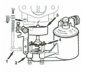
(a) Slacken the jet locking nut (1), using a ring spanner, until the jet bearing (2) is just free to move.
