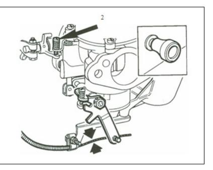
Finally top up the piston damper with thin oil of grade S.A.E. 20 until the level is 12.7 mm (1/2 in) below the top of the hollow piston rod. Mutli-carbs: Remove the air cleaners and carry out items 1, 2 and 3 (single carburettors) on each carburettor.
