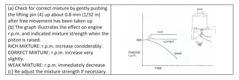
(a) Reconnect the mixture control wire with about 1.6 mm (1/16 in) free movement before it starts to pull on the jet lever.
