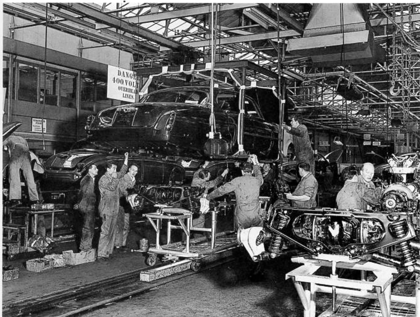
Even though the process was semi-mechanised, the lowering of the massive Mark X body onto its engine and suspension units, still seemed to need at least six pairs of hands. (Jaguar Cars)
