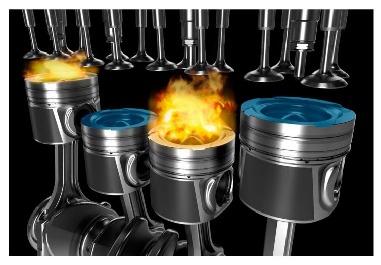
This knock or pinging is the disruption of the delightfully synchronous ballet of sucking, squeezing, banging and blowing - it's upset by virtue of early blowing, which, at high revs and big throttle inputs can destroy your engine. So the designers try to avoid that, sometimes by using a high octane fuel.
