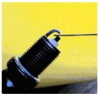
Now adjust gap on whichever spark plug model you are using For a V12 distributor engine, the normal 1.5mm gap must be reset to 0.9mm (0.035"),
