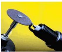
Using a hack saw or dremel, carefully cut the ground electrode at the marking to produce finished result as shown in photo on right.
