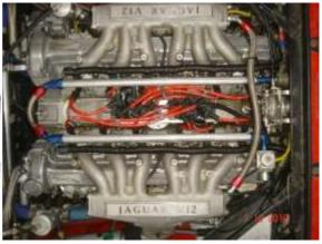
The normal spark plug has the spark igniting inside the plug close to the edge of the head thread; using a projected electrode means the spark is away from the thin edge of the head firing more in the combustion chamber. Together with all my other changes the engine now produces over 400HP.
