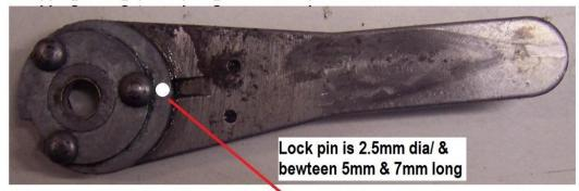
Eccentric cam in park/off possition, 2.5mm hole drilled for a pin to be inserted to lock the cam in place, this will reverse the opperation for a R/H/D so the wiper arms will sweep fully to the bottom of the screen on the drivers side & not the passenger side & park as normal.
